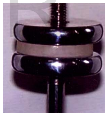
Fig. 8: Plane-Plane Electrode Sample with 8mm gap with Perspex as dielectric medium
