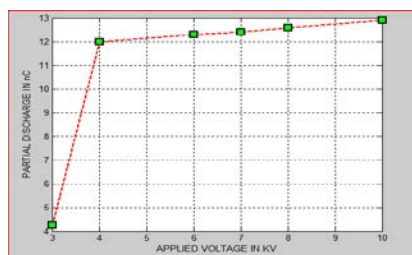
Fig.10: Partial Discharge in nC vs Applied voltage in kV for Solid Insulator –Perspex having dielectric constant 3.5 for Point - Plane Electrode Configuration
